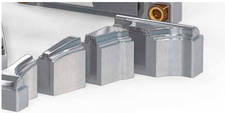
Fig. 3. Illustration of cooling channel design and placement in Press hardening die.
