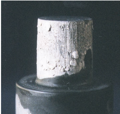
Soldering damage on a core pin.
