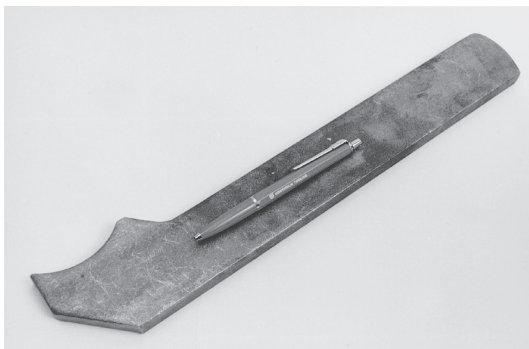
A support arm produced in a blanking tool made from Uddeholm Viking.
