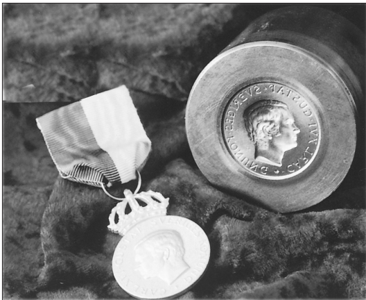
Cold work product where Uddeholm Calmax would be a good choice for the die.
