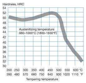
Above tempering curve is obtained after heat treatment of samples with a size of 15 x 15 x 40 mm, cooling in forced air. Lower hardness can be expected after heat treatment of tools, components and dies due to factors like the actual size of the part and heat treatment parameters.
