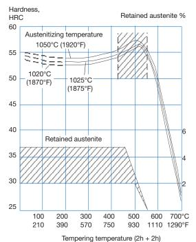
Above tempering curves are obtained after heat treatment of samples with a size of 15 x 15 x 40 mm, cooling in forced air. Lower hardness can be expected after heat treatment of tools and dies due to factors like actual tool size and heat treatment parameters.
