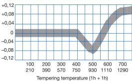
*Note*: The dimensional changes in hardening and tempering should be added.
