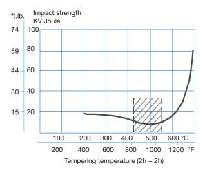
Tempering within the range 425–550°C (800–1020°F) is normally not recommended due to the reduction in toughness properties.
