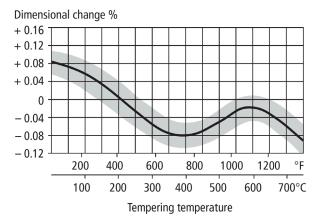
*Note:* Dimensional changes on hardening and tempering should be added together.
