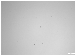
Optical microscope images of polished surfaces and pit density measurements.
