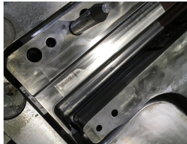
Uncoated W.-Nr. 1.2379 Clear wear marks
