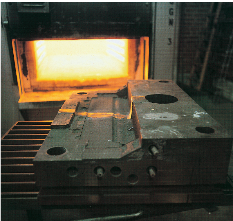
Heat treatment of a die-casting die after welding.
