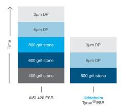
You are able to achieve a high-gloss surface (SPI A1) in three easy polishing steps, resulting in 40-50% less polishing time compared to standard tool steels such as AISI 420 ESR.
