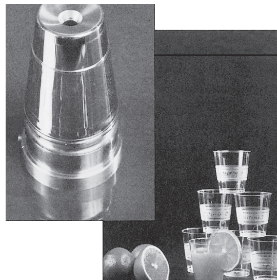
Uddeholm Stavax ESR core to make disposable polystyrene beakers. Millions of close tolerance mouldings with a very high surface finish have been produced.
