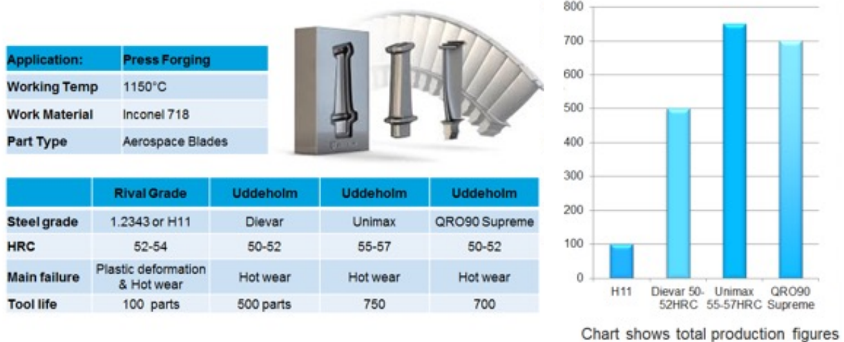
Figure 6 we see the end result of what we have discussed! H11 here gave very limited performance and by uses 3 different Uddeholm problem solvers the company found their best answer with a massive rise in die life.
