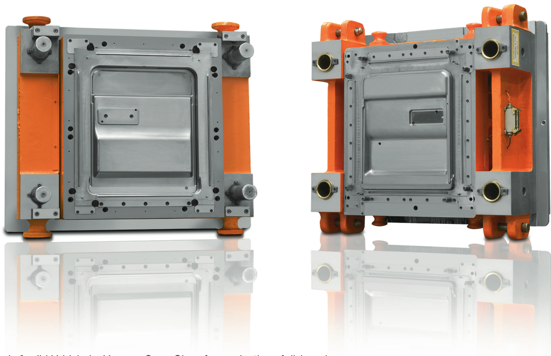
Tool of solid Uddeholm Vancron SuperClean for production of dishwashers.
