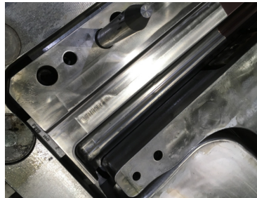
Uncoated W.-Nr. 1.2379 Clear wear marks
