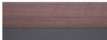
Trimming tool after 100 000 cuts Uddeholm Caldie, 61 HRC, No plastic deformation with Duplex VARIANTIC coating
