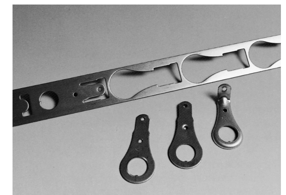
Stainless steel fastener stamped with a Uddeholm Vanadis 23 SuperClean die and Uddeholm Vanadis 4 Extra SuperClean punch.
