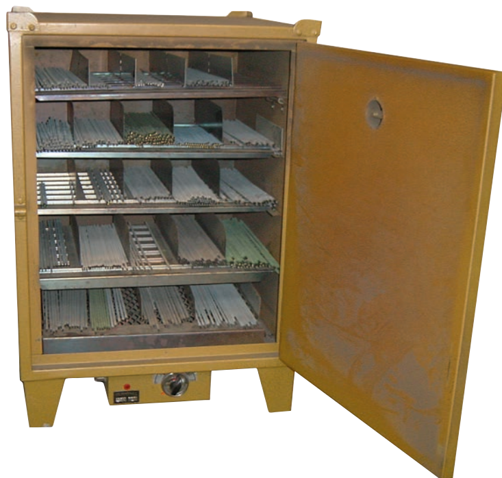
Dry cabinet for storage of electrodes.
